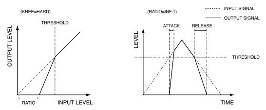
A ducking applies a user-adjustable level of attenuation (RANGE) to input signals that are higher than the threshold level.
