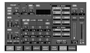
Most screen operations are performed in this area. The name of the current screen is shown in the screen name indication of the top display area. You can use the cursor and function buttons to perform operations in this area.
