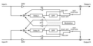
This is a stereo-in, stereo-out cross-modulation delay.
