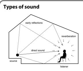
The sound you normally hear is divided into three types: "direct sound," "early reflections," and "reverberation." The "direct sound" is the sound that reaches the listener directly from the source. "Early reflections" are sounds that have reflected one to several times from the walls or other surfaces of the room. "Reverberation" is sound that has reflected many times before reaching the listener.
