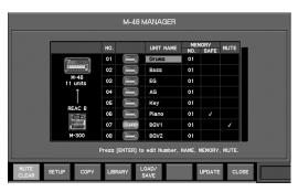
2. In the M-48 list, move the cursor to the desired target M-48 unit and press [F2 (SETUP)].
