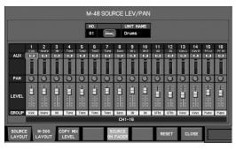
This shows the sources as they are seen from the M-300's fader module section. This display will change according to the M-300's channel layer.
