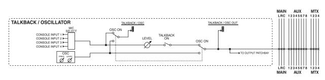
Talkback is a function that sends the input of a mic connected to the CONSOLE IN1–4 on the rear panel jack to an AUX, MTX, MAIN L/R/C, or the output patchbay. This is useful when the mixer operator needs to convey instructions to performers on stage or to staff.
