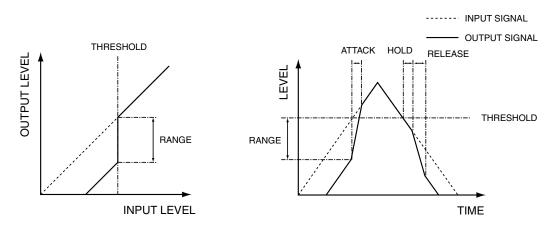
An expander applies a user-adjustable ratio of attenuation (RATIO) to input signals that are lower than the threshold level.
