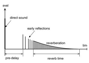
The reflected sounds reach the listener in the following order. The pre-delay is the time from when the direct sound is heard until the reverb arrives. The reverb time is the duration until the reverb disappears.
