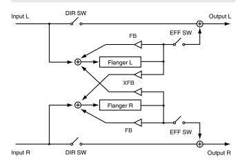
This is a stereo-in, stereo-out flanger. It lets you apply flanging without impairing the position of the sound image that's been set for the stereo input, by panning or other means.
