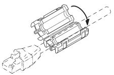
4. Connect the plug with the ferrite core to the M-300's REAC port.
