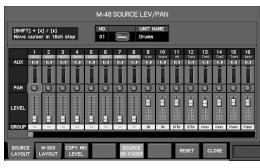
This shows the sources arranged in order of their number (the order in the M-300's REAC B output patchbay).
