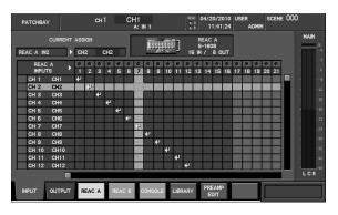
2. Press [F2 (OUTPUT)] and [F4 (REAC B)] to view the REAC B output patchbay.
