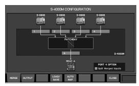
If the "Split Inputs to PORT4" button in the PORT4 OPTION is checked, then the S-4000M's split function is already turned on. The following steps will not be necessary.
