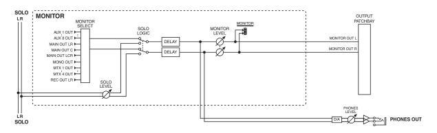
Monitoring is a function by which the AUX, MTX, MAIN, or USB memory recorder signal that you select as the monitor source can be sent from the output jacks or headphone jack. This is used mainly by a mixing engineer to monitor the signals.
