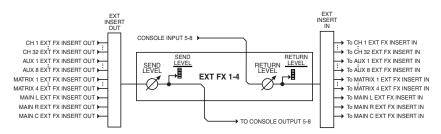
You can use the CONSOLE IN 5–8 and CONSOLE OUT 5–8 jacks located on the M-300's rear panel to insert up to four external effects devices into channels. The four external effects devices are shown virtually as an EXT FX1–EXT FX4 rack, allowing you to adjust the input levels and insert them into channels.
