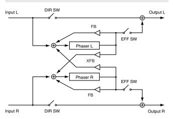
This is a stereo-in, stereo-out phaser. It lets you apply a phaser effect without impairing the position of the sound image that's been set for the stereo input, by panning or other means.
