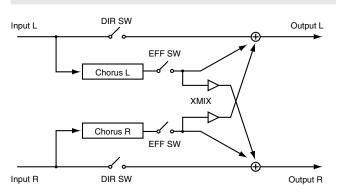
his is a stereo-in, stereo-out chorus. It lets you apply chorus without impairing the position of the sound image that's been set for the stereo input, by panning or other means.
