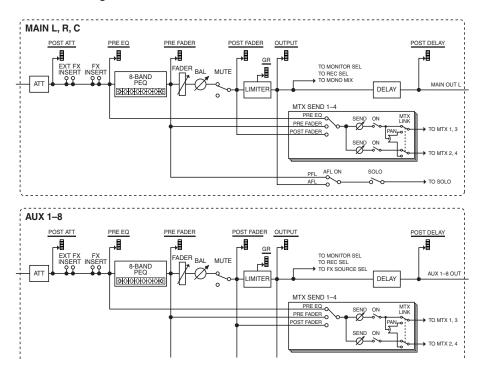
The MTX sends are used to send audio signals from AUX1-8 or MAIN L/R/C to MTX1-4.
