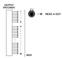
When the M-300's REAC is set to MONITOR/BROADCAST (p. 140), the REAC A port operates as the REAC split. In this case, the M-300 cannot output signals to the REAC A.
