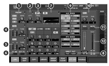
The principal operations for an input channel can be performed in the CHANNEL DISPLAY screen.
