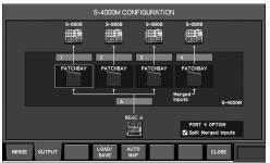
5. Connect the REAC cable to REAC port 4 on the S-4000M.
