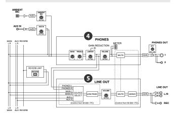
The M-48 provides two sets of output: PHONES and LINE OUT.
