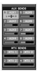
Here you can adjust the sends from the channel to the AUX1–8 or MTX1–4 buses.
