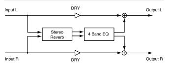
This is a stereo-in, stereo-out reverb. It adds reverberation without impairing the position of the sound image that's been set for the stereo input, by panning or other means.
