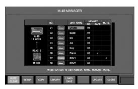
2. In the M-48 list, move the cursor to the UNIT NAME of the desired M-48 and press [ENTER].
