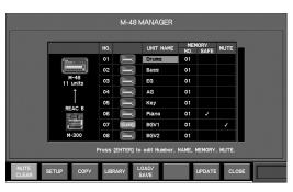
2. In the M-48 list, move the cursor to the desired copysource M-48 unit, and press [F3 (COPY)].
