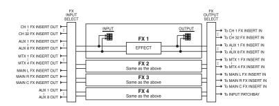
The M-300 contains four internal effects (FX1–FX4), each of which allows you to select from 11 different effect types including reverb, delay, and 31-band GEQ.
